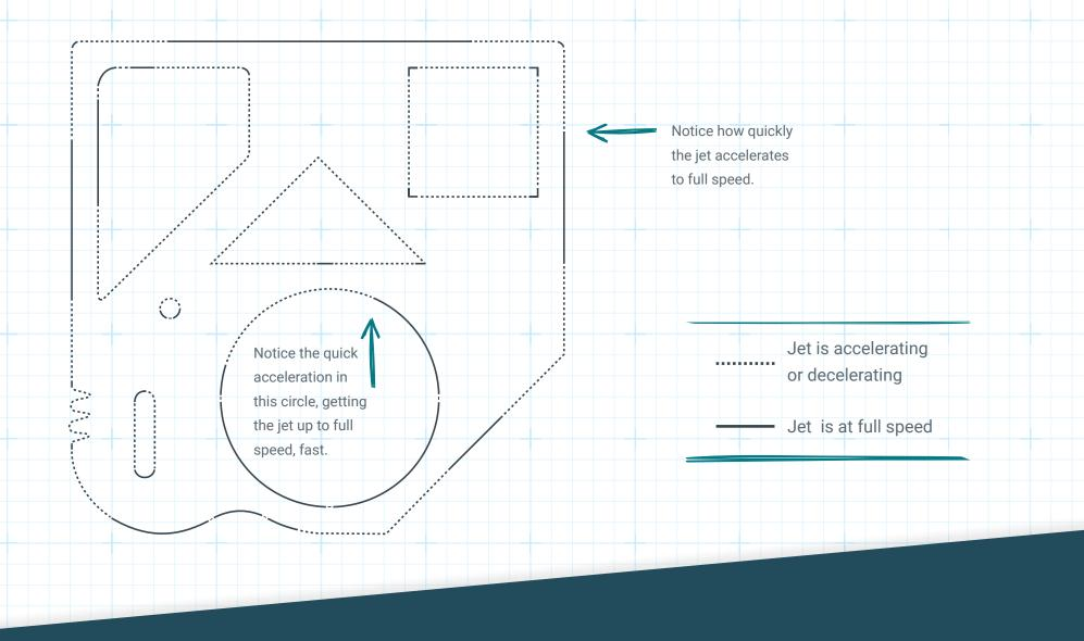
**WATERJET PARTS** are generally made up of diverse geometry, therefore you rarely find yourself cutting at top speed. This sample part visually demonstrates why a fast acceleration and deceleration speed is important to your overall cut part productivity.
