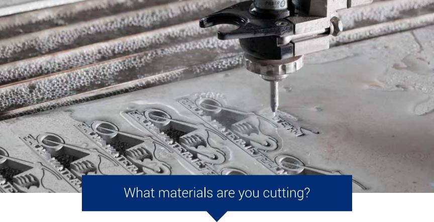
The first step in determining the right waterjet is to define the kinds of materials you work with or plan to work with in your operation. When it comes to materials, the major considerations are: current and potential future material types, material stock size, material thickness, and part shape (flat, bevel, or 3D).
