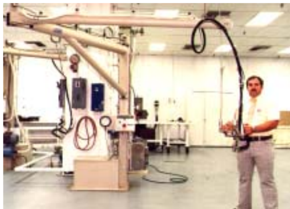
Handheld "Universal WaterRouter." A point catcher safely stops the jet immediately after cutting the thin material.
