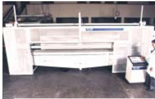
Cross Cutter - usually angled across and timed with the travel path of the product. Precise speed control can then produce a perpendicular cut.
