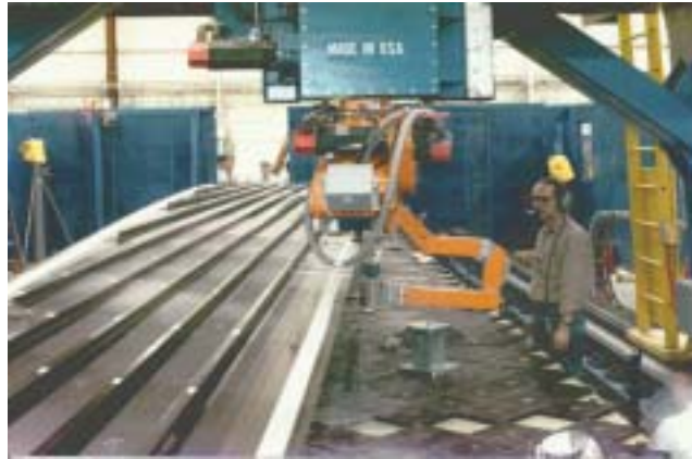
This 3D Machine Tool with a 5-axis wrist uses swivels to provide movement of the head. This particular machine employs a point catcher to catch the jet. Cutting of aerospace composites.
