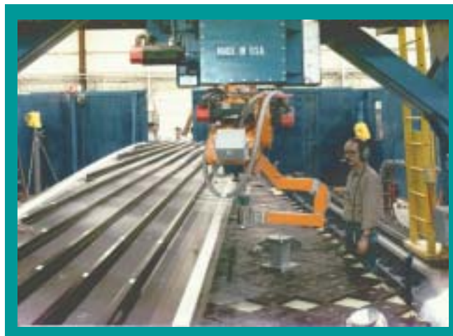
C-frame holds the unique point catcher. This catcher can stop a 50 HP abrasive Waterjet in just 6 inches. A vacuum constantly removes the slurry.
