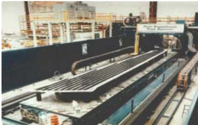
A large 30x15x4 ft. machine cuts tail components for the Boeing 777. "Pogostick" tooling unscrews to specified height, then vacuum cups hold the part in place.
