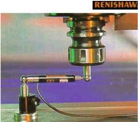
The telescoping Ballbar is ready to begin recording. The machine will execute a circle around the base and errors will be recorded.
